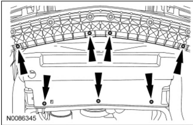
3. Remove the 6 pushpin retainers and the air deflector.
